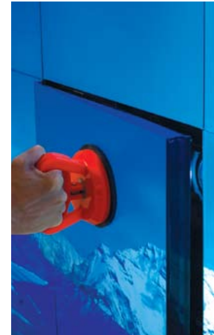
A handy suction cup provides quick and easy access to any tile in an array.
